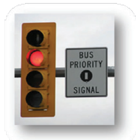
Bus Priority Signal Similar to Contemporary Signals Except for Additional Light
